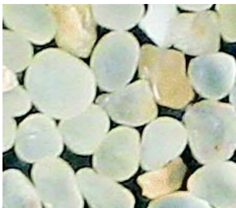
Figure 3 – 1 Photograph of the spherical grains of the 12/20 sand. [DiCarlo 2004]
