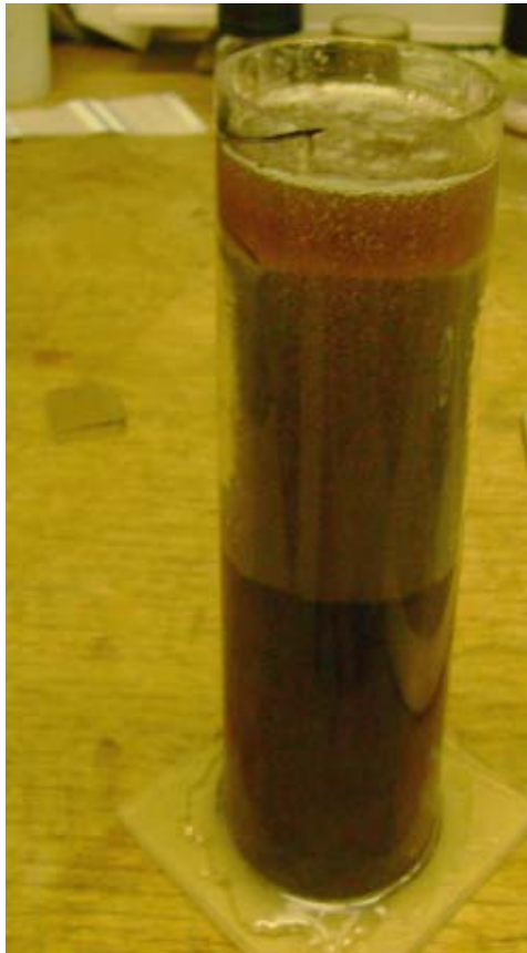
Figure A3: The plastic tube containing shale and filler rock, filled with epoxy.
