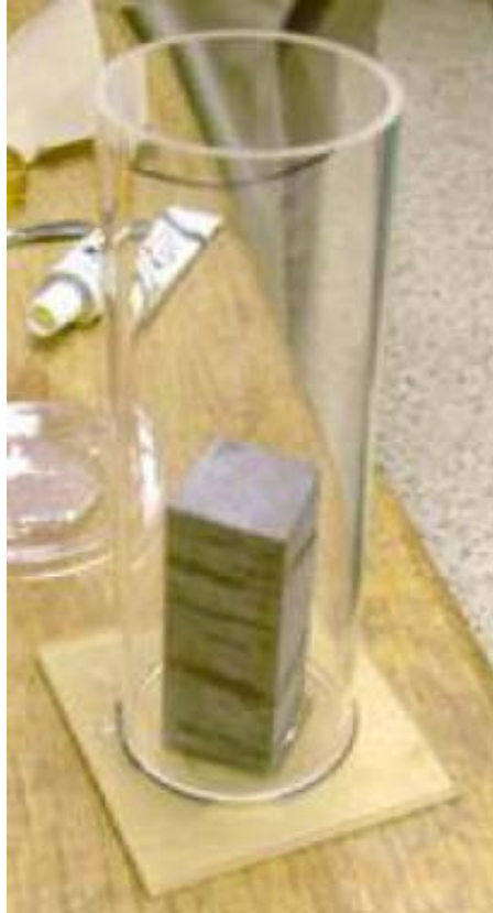
Figure A2: Plastic tube placed on a base covering the shale column.
